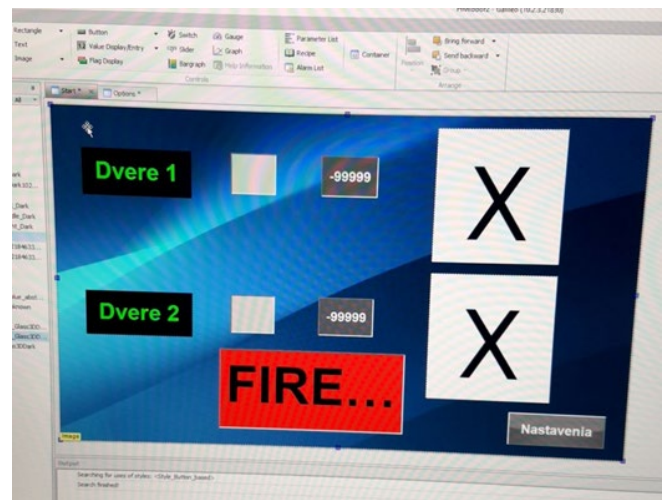
Fig. 4. Programming application for PLC/HMI Eaton XV1xx.
