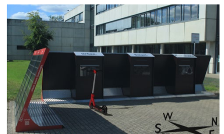
Fig. 2. Off-Grid Solar charging station installed by the Sustainable Technology Laboratory on the campus of Bochum University of Applied Sciences.
